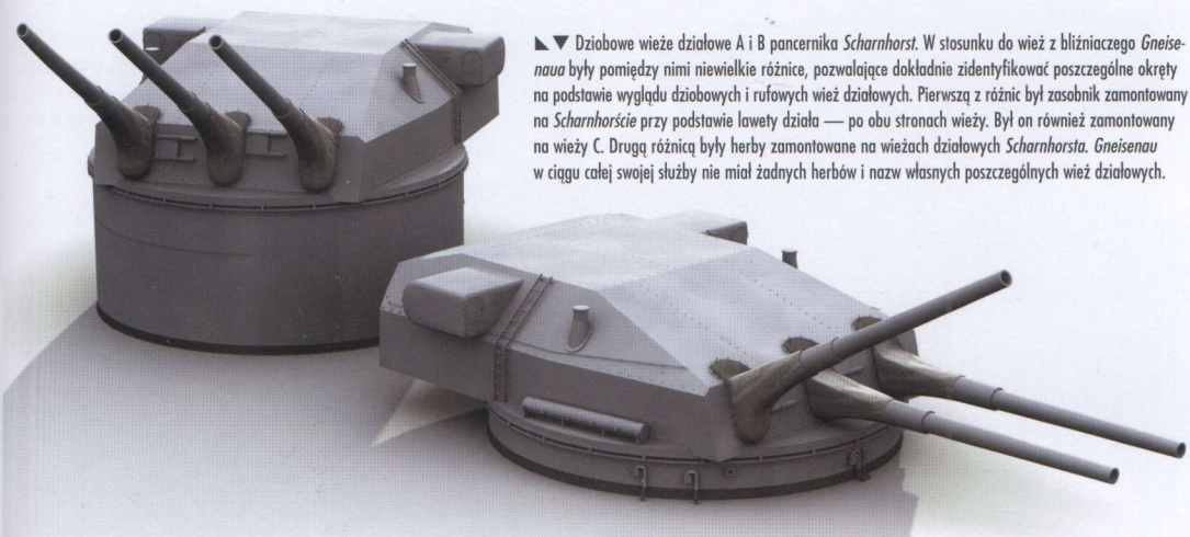
▼ Forward main battery gun turrets A and B of the battleship Gneisenau after commission. The L C/34 turret was generally identical to the Deutschland -Class L C/28, except for a thicker armor.
