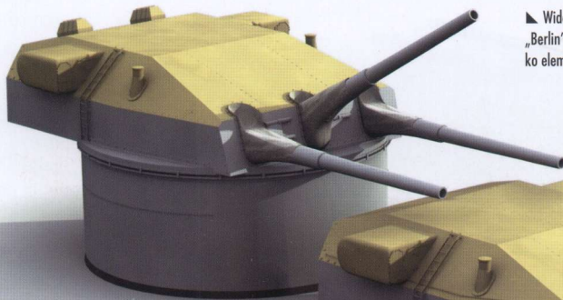
► Right side view of the A and B turrets and B turret bar-bette of the Scharnhorst during Operation Berlin, when roofs and top slopes of the gun turrets were painted yellow as a quick identification sign for the German air force.
